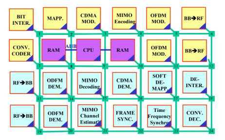
Figure 4: Function mapping topology on NoC
