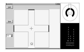
**Figure 2** Left: the robot in the plus maze environment. A white arm extremity indicates the reward location. Other arm extremities do not deliver any reward and are shown in black. Upper right: the robot's visual perceptions. Lower right: activation level of different channels in the model.
