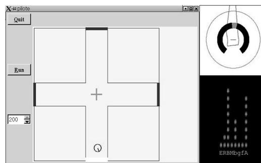
**Figure 2** Left: the robot in the plus maze environment. A white arm extremity indicates the reward location. Other arm extremities do not deliver any reward and are shown in black. Upper right: the robot’s visual perceptions. Lower right: activation level of different channels in the model.
