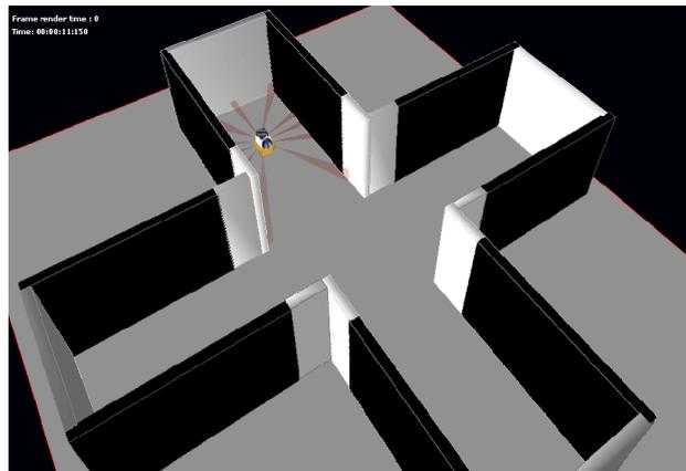
**Figure 8** Simulation of the plus-maze task in a 3D environment. Like the 2D environment, one random arm extremity is white and delivers reward. The animat has to perform taxon navigation so as to find and consume this reward. Grey stripes arising from the animat’s body represent its sonar sensors used by its low level obstacle avoidance reflex.
