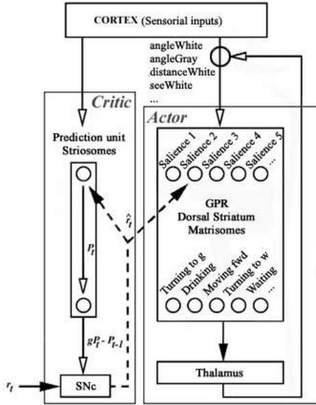
**Figure 3** The Actor-Critic model of reinforcement learning. The Actor module is a GPR model that is segregated in different channels, with saliences as inputs and actions as outputs. The Critic module (involving striosomes in the dorsal striatum or in the nucleus accumbens shell, and the substantia nigra compacta (SNc) (or ventral tegmental area (VTA))) propagates towards the actor module an estimate  $\hat{v}$  of the instantaneous reinforcement triggered by the selected action.
