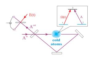
FIG. 1: (Color online) Quantum memory set-up: field  $A^{in}$  is sent into a cavity containing an ensemble of three-level atoms. The coupling of the intracavity field A(t) with the atomic ground state variables is dynamically controlled by a pulsed coherent field  $\Omega(t)$ . The fluctuations of the output field  $A^{out}$ are measured by homodyning with a local oscillator E(t), the temporal profile of which may be adjusted so as to optimize the detection efficiency.
