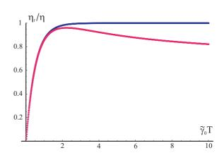
FIG. 4: (Color online) Readout efficiency  $\eta_r$  (normalized by the *cw* efficiency  $\eta$ ) versus pulse "area"  $a(\infty) = \tilde{\gamma}_0 T$  when the LO is either the retarded readout pulse (lower curve) or a pulse temporally matched with the atomic emission (upper curve).
