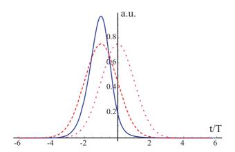
FIG. 3: (Color online) Radiated pulse (plain), read pulse (dotted) and delayed read pulse (dashed) envelopes vs time t/T, for  $\tilde{\gamma}_0 T = 5$ .
