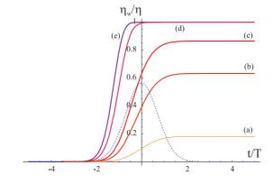
FIG. 2: (Color online) "Write" efficiency  $\eta_w(t)$  (normalized to  $\eta$ ) versus time t/T, when the write pulse "area" increases [Gaussian envelopes with (a)  $a(\infty) = 0.1$  (b) 0.5 (c) 1 (d) 5 (e) 10]. The dashed curve represents the write pulse envelope  $\xi(t)$ .
