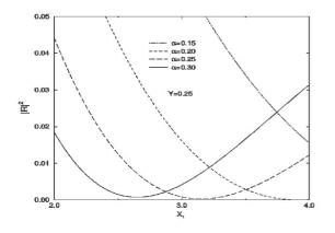
**Figure 3** : Broadband antireflection properties of a thin film, coating a lossy dielectric with  $n_2 = 3.5$ ,  $\chi_2 = 0.7$ ; the dependence of the reflectivity  $|\mathbf{R}|^2$  upon the normalized frequency  $x_1 = \omega/\Omega_1$ , relating to the case y = 0.25,  $n_0 = 1.6$ ,  $p^2 > 0$ ,  $s_2 < 0$ , is represented for different values of the parameter  $\alpha = d/L_2$ . The same dielectric without coating has a reflection coefficient  $|\mathbf{R}|^2 = 0.32$
