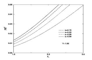
**Figure 1**: Antireflection properties of thin inhomogeneous dielectric film in the case  $s_2 < 0$  and  $p^2 > 0$  (8). The reflection coefficient  $|\mathbf{R}|^2$  is plotted vs the normalized frequency  $x_1 = \omega/\Omega_{I_1}$  for  $n_0 = 1.73$ , and for different values of the parameter  $\alpha =$
