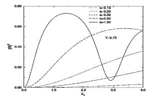
**Figure 2** : Spectra of reflectivity of inhomogeneous film in a case  $s_2>0$  and  $p^2 < 0$  (8); The reflection coefficient  $|\mathbf{R}|^2$  is plotted vs. the normalized frequency  $x_2 = \omega/\Omega_2$  for  $n_0 = 1.73$ , and for different values of the parameter  $\alpha = d/L_2$ .
