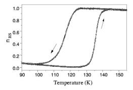
FIG. 1. Thermal hysteresis [high-spin fraction ( $n_{\rm HS}$ ) vs temperature] of Co(H<sub>2</sub>(fsa)<sub>2</sub>en)(py<sub>2</sub>), obtained by reflectivity measurements.
