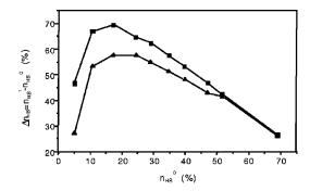
FIG. 5. Comparison of the amplitudes of conversion in  $Co(H_2(fsa)_2en)py_2$  obtained experimentally (triangles) and by using the quasistatic approach (squares).
