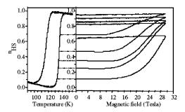
FIG. 4. Set of isotherms  $n_{\rm HS}(B)$  showing the irreversible (and quasitotal) triggering effect on the HS fraction in  ${\rm Co(H_2(fsa)_2en)(py)_2}$  for an applied PMF in the metastable LS state.
