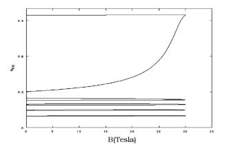
FIG. 7. Calculated HS fraction as a function of the pulsed magnetic field **B** in the ascending branch of the hysteresis loop.
