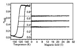
FIG. 3. The reversible response of a HS fraction in  $Co(H_2(fsa)_2en)(py)_2$  to an applied PMF in the metastable HS state.
