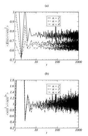
Fig. 3. Nonlinear oscillator with additive, colored noise: equations (45–46) are integrated numerically for  $\mathcal{D}=1$  and  $\tau=1$ , with a timestep  $\delta t=10^{-6}$  and averaged over 500 realizations for n=2,3,4. (a) The first equipartition ratio  $\langle E(t)\rangle/\langle v(t)^2\rangle$  is close to the theoretical value  $\frac{n+1}{2n}$  given in equation (20). (b) The second equipartition ratio  $\langle v(t)^2\rangle/\langle x(t)^{2n}\rangle$  is close to 1.
