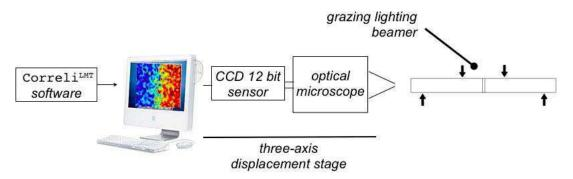
Figure 5. Schematic of the testing procedure using a DIC technique.
