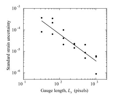
Figure 3. Standard strain uncertainty for different gauge sizes when l = 64 pixels and  $\delta = 32$  pixels. The straight line shows a power law fit with an exponent of -1.25.
