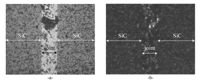
Figure 4. Digital images  $(1280 \times 1024 \text{ pixels}, 1 \text{ pixel} = 0.33 \mu\text{m})$  acquired with a normal lighting beam (a) and a grazing lighting beam (b).
