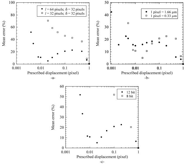
Figure 2. Performance in terms of mean error vs. prescribed displacement for different correlation parameters (a), magnifications (b) and digitizations (c).
