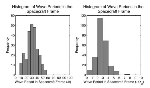
**Figure 5.** Histogram of wave periods observed in the spacecraft frame over 255 samples. The waves are quasi-monochromatic in the individual cases. The left-hand panel shows the raw data. The variation about the average is significantly larger than the experimental error in each observation. The right-hand panel is scaled to the local proton gyrofrequency.
