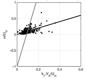
**Figure 7.** Plot of plasma frame wave frequency normalized by  $\Omega_{ci}$  against parallel wave number, normalized by  $\Omega_{ci}/V_A$ , for each of 255 subintervals of monochromatic ULF wave activity. The experimental error in  $\Omega_{ci}/V_A$  is ~20– 40%. The black line corresponds to the Alfvèn speed. Clustering of the data is seen, as might be expected from Figure 2. The gray line, based on the mean values of frequency and wave number, represents the beam resonance condition.
