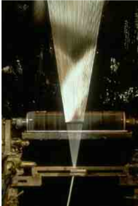
Fig. 5: a multipurpose aqueous dispersion (sizing) is applied to the glass filaments before they are pulled together to form a reinforcement fiber. Among other properties, the sizing lubricates the fiber contacts to reduce surface flaw generation. Copyright Saint-Gobain.
