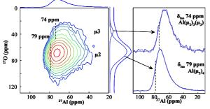
*Figure 3* :  $\{^{17}O\}^{27}AI$  HMQC spectrum ( $v_R 25$ kHz,  $\tau 7$ ms, 17.6T, 480 scans) of CA-glass ( $^{17}O 30\%$  enriched ) and  $^{27}AI$ -slices taken at  $\mu_2$  and  $\mu_3$  locations, exhibiting a 5 ppm difference in the isotropic chemical shift. The doted lines are the modelled lines considering a GIM distribution<sup>2</sup>. The dashed lines indicate the position of <sup>27</sup>Al isotropic chemical shifts.
