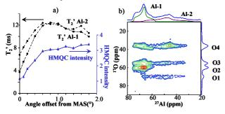
Figure 2 : <sup>17</sup>O 30% enriched CA2-CaAl<sub>2</sub>O<sub>7</sub> crystalline sample : a) variation of T2' for the two Al sites and HMQC intensity (normalized to on angle) versus angle offset from MAS. b) {<sup>17</sup>O}<sup>27</sup>Al HMQC spectrum (v<sub>R</sub> 15kHz, τ 3ms, 17.6 T-750 MHz, 64 scans).
