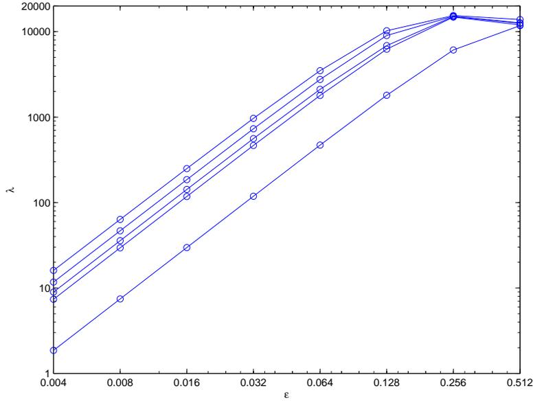
Figure 3: First 5 eigenvalues plotted against  $\varepsilon$ , load L3
