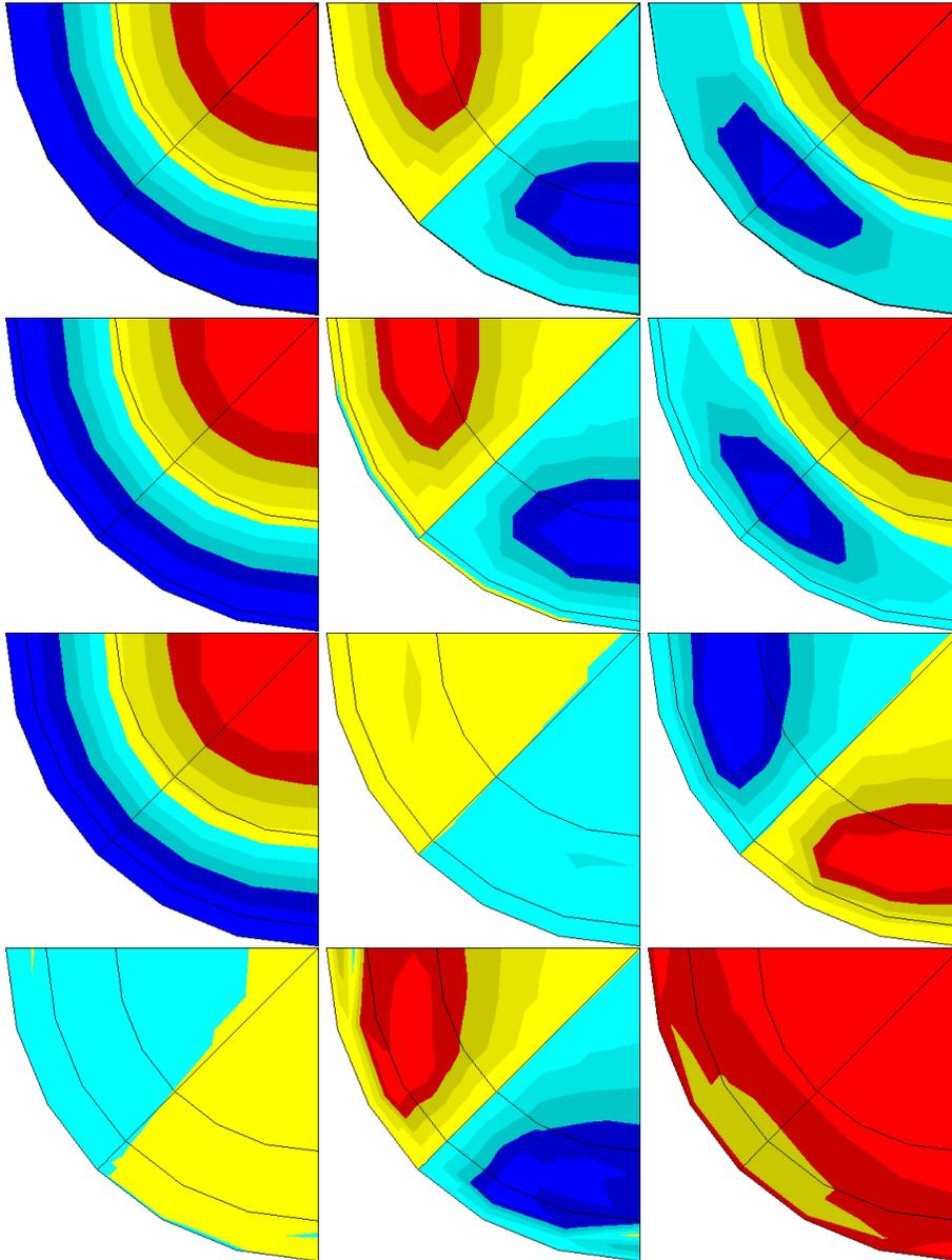
Figure 4: Midplane plot of  $u_3$  for first three eigenvectors, load L3, mesh MID.
