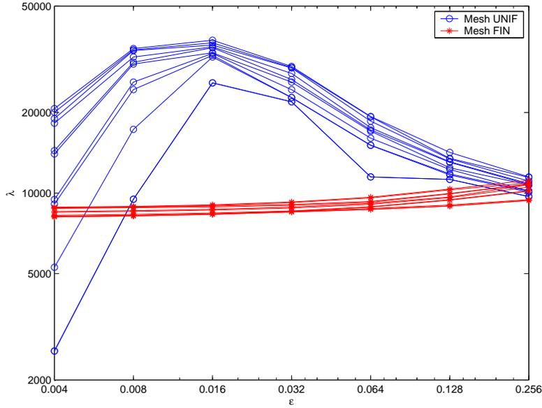
Figure 2: First 10 eigenvalues plotted against  $\varepsilon$ , load L1
