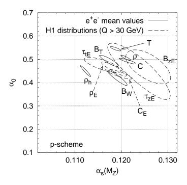
Figure 1.  $\alpha_s(M_Z^2)$  and  $\alpha_0$  from jet shapes. 1– $\sigma$  contours for the means in  $e^+e^-$  annihilation (solid) and for the shape distributions in the current fragmentation jet in DIS (dashed).
