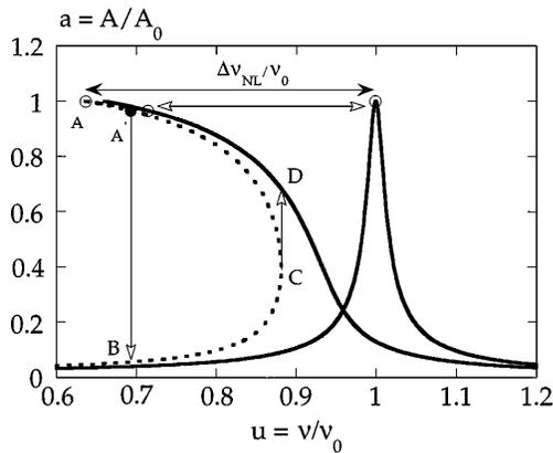
FIG. 2. Shifts in resonance frequency  $\Delta v_{NL}$  correspond to shifts given by the black arrows. Because of the experimental uncertainties and the flatness of the distorted curve (Fig. 1), even with a constant amplitude mode various situations can occur. If the oscillator is trapped on the lower instable curve (black circle on the dotted line), then a cycle of hysteresis following the path  $A'BCD$  follows.
