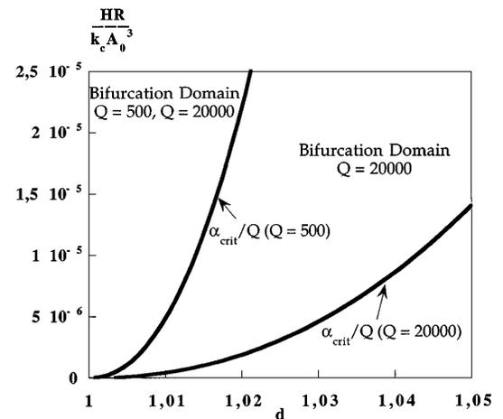
FIG. 3. Determination of the domain of bifurcation calculated for two values of the quality factor  $Q$ . The curves are calculated with the equation given in Ref. [22]. The curves  $\alpha_{crit}/Q$  give the frontier above which the resonance peak starts to distort.
