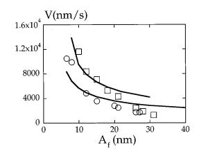
FIG. 9. Observed growth rates compared to the numerical results. Empty circle  $M_w = 95000$ , empty square  $M_w = 23000$ . The parameters are  $J_0F_{\text{ext}} = 20 \text{ nm}$ ,  $\tau_N = 143 \times 10^{-6} \text{ s}$ ,  $d_c = 4 \text{ nm}$ , and  $J_0F_{\text{ext}} = 8 \text{ nm}$ ,  $\tau_N = 67 \times 10^{-6} \text{ s}$ ,  $d_c = 3 \text{ nm}$ , respectively, for  $M_w = 23000$  and  $M_w = 95000$ .
