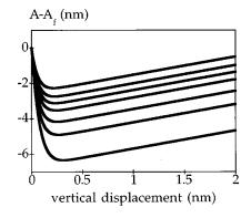
FIG. 7. Results of the numerical simulations using Eqs. (12), (13), and (14). The parameters are  $J_0 F_{\text{ext}}=15 \text{ nm}$ ,  $\tau_N=143 \times 10^{-6} \text{ s}$ , and  $d_c=3 \text{ nm}$ . From the lower to the upper curve the starting amplitudes are 8, 10, 12, 15, 18, 22, and 30 nm.
