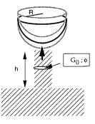
FIG. 5. Sketch of a nanoprotuberance created under the action of a oscillating nanotip. The geometry of the nanoprotuberance is the simplest one: a cylinder of diameter  $\phi$  and height *h*.  $G_0$  is the associated elastic modulus. *R* is the radius of the tip.
