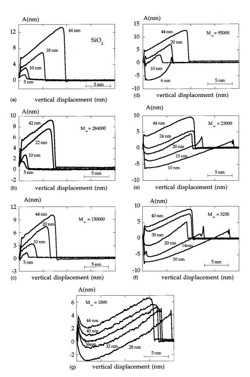
FIG. 3. Variations of the amplitude of the oscillation during the retraction of the surface as a function of the free amplitudes  $A_f$  for different samples. Scan size 20 nm, scan frequency 10 Hz.
