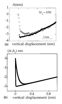
FIG. 8. Zoom of the fast part of the variation of the oscillating amplitude for two velocities of the piezoactuator. (a) Experimental data  $M_w$ =3250 and  $A_f$ =20 nm. Empty symbol  $v_p$ =400 nm/s, filled symbol  $v_p$ =20 nm/s. (b) Numerical simulation with the parameters  $J_0F_{\rm ext}$ =14 nm,  $\tau_N$ =143×10<sup>-6</sup> s,  $d_c$ =3 nm and the starting amplitude 15 nm.
