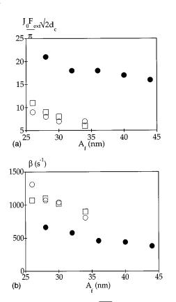
FIG. 11. Parameters  $(J_0F_{\rm ext}/\pi)\sqrt{2d_c}$ . (a) and  $\beta$  (b) calculated from the fits shown in Fig. 10. The parameters  $\alpha$  remain constant:  $\alpha = 0.25$  (2)  $(M_w = 1890)$ ,  $\alpha = 0.53$  (2)  $(M_w = 3250)$ ,  $\alpha = 0.50$  (1)  $(M_w = 23\ 000)$ . Filled circle,  $M_w = 1890$ ; empty circle,  $M_w = 3250$ ; empty square,  $M_w = 23\ 000$ .
