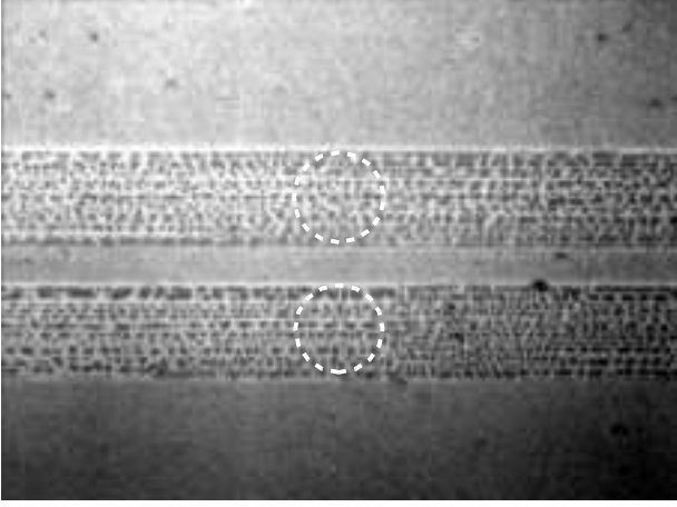
Fig. 6. Breath figure formed on exposing to water-saturated air a bare glass surface onto which a PMMA lens has slid along two parallel tracks. A continuous wetting film forms over clean glass, whereas a droplet pattern decorates the two tracks. The dashed circles indicate the size of the contact zone for both tracks. Image size is 615 \times 455 \mu\text{m}^2 .
