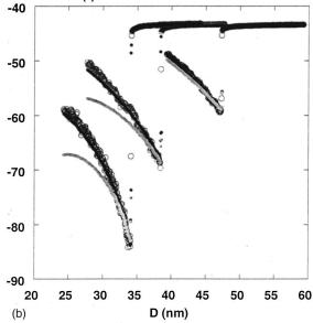
FIG. 7. Variations of the phase in intermittent contact situations for different working amplitudes. A comparison with calculated curves: Black dots power law  $A^{-2}$ , Eq. (10b); gray dots power law  $A^{-5/2}$  [Eq. (7a)]. Silica surface,  $A_{\rm free}$ : 35, 31, 22, 18 nm (Fig. 8a), APTES surface  $A_{\rm free}$ : 44, 35, 31 nm (Fig. 8b).
