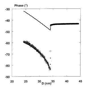
FIG. 6. Example showing the influence of the noncontact dissipation for the intermittent contact situation. The continuous line is obtained by calculating the phase with  $\phi = \sin^{-1}(uA/A_0)$  [Eq. (7b)], the filled circles are given by a fit with Eq. (10b). The experimental data (open circle) correspond to the APTES surface with  $A_{\rm free} = 31$  nm.
