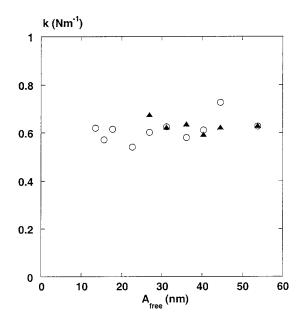
FIG. 8. Variation of the mechanical susceptibility k of the surface controlling the amount of noncontact dissipation. The values are obtained from fits with Eq. (10b) (see Fig. 7) with  $\Delta$ =0.5 nm. Open circle: silica surface; filled triangle: grafted surface.
