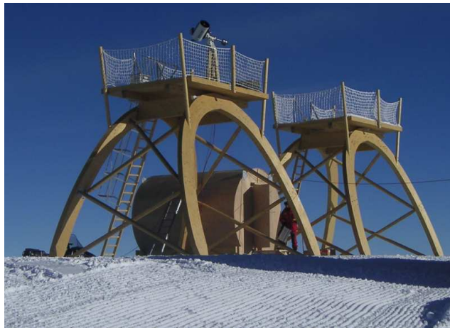
Fig. 1. Concordiastro observatory in November 2004. One can see the two platforms and the wooden igloo between. The DIMM is on the top of one platform.
