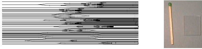
Fig. 8. Mask produced with LEMO facilities containing tests components for telescope beam combination (2, 3 and 4 telescope) either in coaxial and multi-axial mode (left). Half part of the chip (right), contains all the components.
