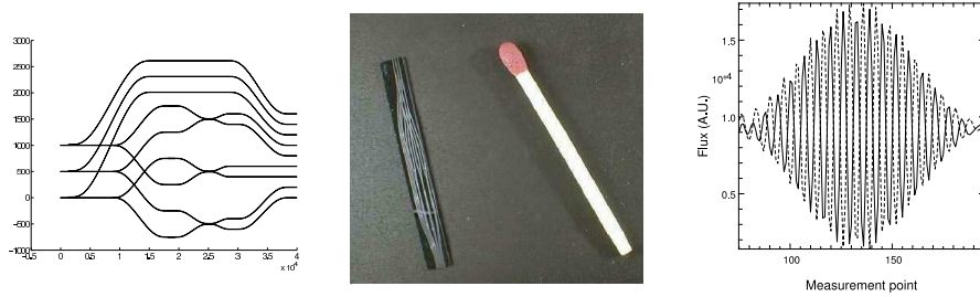
Fig. 7. 3 telescope beam combiner produced using LETI facilities. Beam combiners are asymmetrical couplers optimized for the whole H band [30]. The obtained interferograms show 90% contrast through the H band, and a throughput higher than 60%
