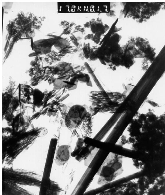
Fig. 4. TEM image of powder derived from hydrothermal treatment of **Y5**.
