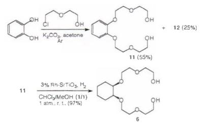
Fig 10. Synthesis of 1,2-bis(5-hydroxy-3-oxapentyloxy)cyclohexane cis 6.
