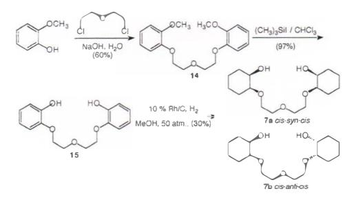
Fig 14. Synthesis of 2,2'-[3-oxapentane-1.5-diylbis(oxy)diyl]dicyclohexanol cis 7a and 7b.
