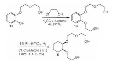
Fig 13. Synthesis of 1-(5-hydroxy-3-oxapentyloxy)-2-(2-hydroxyethoxy)cyclohexane cis 5.
