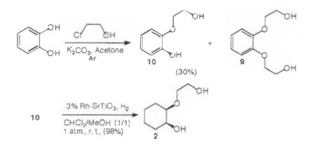
Fig 8. Synthesis of 2-(2-hydroxyethoxy)cyclohexanol cts 2.
