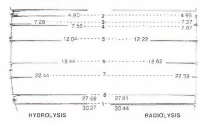
Fig 3. Comparison of radiolysis and hydrolysis chromatograms.
