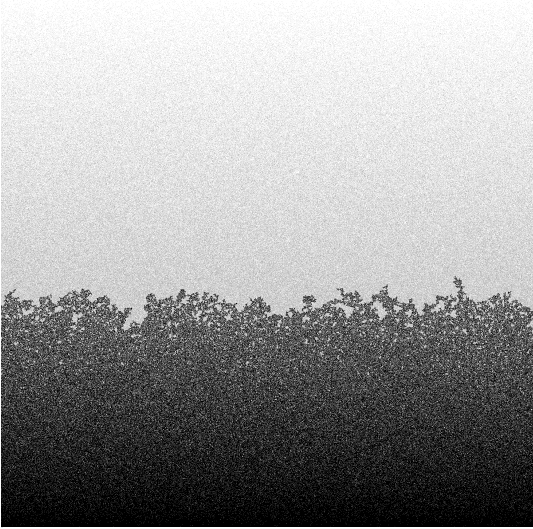
Figure 5: Gradient percolation in a square. In black is the cluster spanning from the bottom side of the square.
