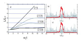
Figure 4: a) Time evolution of the rms size L of the BEC in the random potential V for various values of the speckle amplitude  $\sigma_V = \gamma \mu$  and comparison to the theoretical prediction in the absence of random potential (black dotted line). b-c) Density profiles of the BEC trapped by disorder at two different times  $\omega_z t = 10$  and  $\omega_z t = 20$  respectively.
