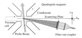
Figure 2: Optical setup used to create the random speckle potential. The long axis of the condensate is oriented along the z direction.
