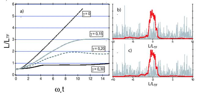
Figure 4: a) Time evolution of the rms size  $L$  of the BEC in the random potential  $V$  for various values of the speckle amplitude  $\sigma_V = \gamma\mu$  and comparison to the theoretical prediction in the absence of random potential (black dotted line). b-c) Density profiles of the BEC trapped by disorder at two different times  $\omega_z t = 10$  and  $\omega_z t = 20$  respectively.
