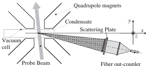
Figure 2: Optical setup used to create the random speckle potential. The long axis of the condensate is oriented along the  $z$  direction.
