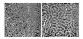
FIG. 1: Intermediate state pattern on the edge of the  $10 \ \mu m$  thick superconducting Indium slab for h=0.07 (left) and h=0.41 (right) at T=2 K. The edge of the In slab is along the right edge of the images. Normal and superconducting domains appear in black and gray, respectively. The few white domains correspond to magnetic flux which was trapped at h=0 (details on image processing are given in Ref. [20]).
