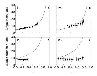
FIG. 2: Mean lamella width W (top) and bubble diameter 2R (bottom) as a function of the reduced field  $h=H/H_c$  for a  $10~\mu m$  thick In slab (left) and a  $120~\mu m$  thick Pb slab (right). The error bars represent the full width at half maximum of the distributions of lamella width or bubble diameter. The solid lines are the equilibrium values  $2R_{eq}$  and  $W_{eq}$ .
