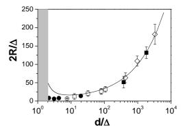
FIG. 3: Semi-log plot of the reduced bubble diameter  $2R/\Delta$  versus reduced sample thickness  $d/\Delta$ . The filled circles and squares were obtained with In and Pb slabs, respectively. The empty squares, lozenges and circles are reported from Ref. [14, 15, 16], for Pb, Hg and In, respectively. The gray region corresponds to Type-II superconductivity for very thin slabs. The solid curve is the equilibrium diameter (Eq. 2).
