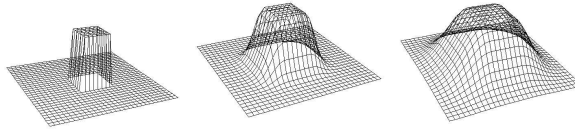
Figure 2: The distribution corresponding to inequality constraints induced by a Point-On-Face relationship for a square face at different values of temperature. The left figure shows the original constraints ( T = 0 ), while the middle and the right ones show these constraints relaxed at ( T = 50 ) and ( T = 100 ) respectively.
