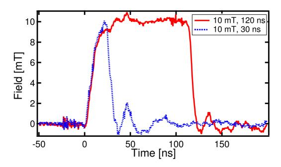
Figure 1: Shape of the magnetic field pulses. Solid and dotted curves correspond to 120 ns and 30 ns pulses, respectively. The height of both pulses shown here is 10 mT.
