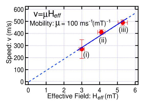
Figure 4: Domain wall speed as a function of effective field extracted from Fig. 3. The effective field was obtained by addition or subtraction of the pulse field and coupling field (2.0 mT) for configurations B and A, respectively. Mobility  $\mu$  of the wall motion was obtained by a linear fit to  $v=\mu H_{eff}$ , which resulted in 100 m s<sup>-1</sup>(mT)<sup>-1</sup>.
