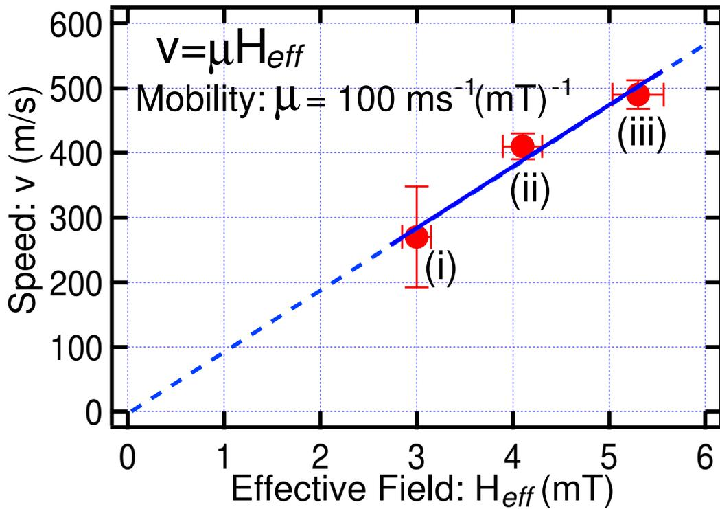
Figure 4: Domain wall speed as a function of effective field extracted from Fig. 3. The effective field was obtained by addition or subtraction of the pulse field and coupling field (2.0 mT) for configurations B and A, respectively. Mobility  $\mu$  of the wall motion was obtained by a linear fit to  $v = \mu H_{eff}$ , which resulted in  $100 \text{ m s}^{-1}(\text{mT})^{-1}$ .
