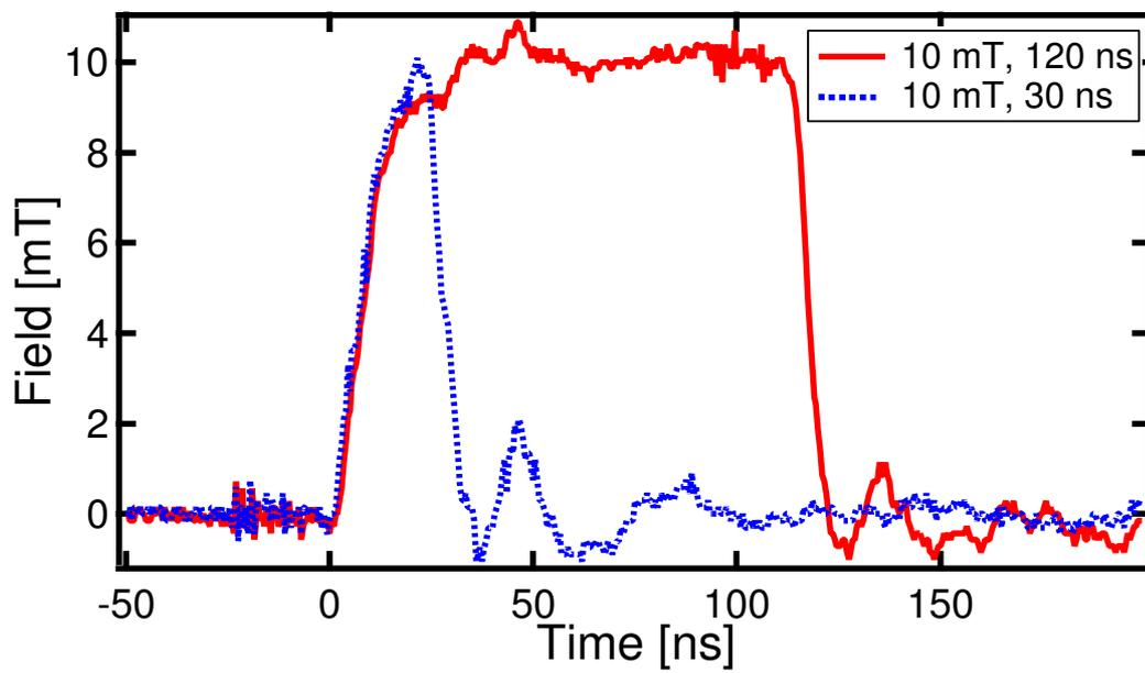
Figure 1: Shape of the magnetic field pulses. Solid and dotted curves correspond to 120 ns and 30 ns pulses, respectively. The height of both pulses shown here is 10 mT.
