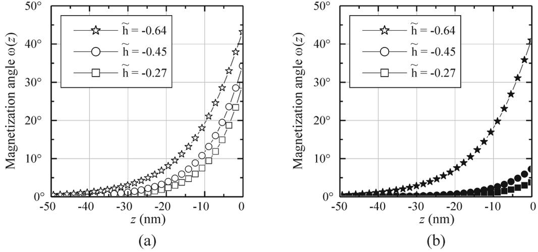
Fig. 6. Magnetization angle  $\omega(z)$  predicted by the model in a dot of thickness  $27 \text{ \AA}$  for several applied magnetic fields: In (a) the edge direction is  $\beta = 70^\circ$  and  $\tilde{h}_r = -0.75$ , and in (b)  $\beta = 89^\circ$  and  $\tilde{h}_r = -0.66$ . Physical parameters are:  $A = 2 \times 10^{-11} \text{ J.m}^{-1}$ ,  $M_s = 1.73 \times 10^6 \text{ A.m}^{-1}$ ,  $K = 4.76 \times 10^5 \text{ J.m}^{-3}$ .
