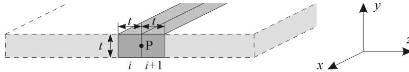
Fig. 9. Schematic illustration of the two in-plane cylinders  $i$  and  $i+1$  of section  $t \times t$  taken into account to estimate the strength of dipolar fields arising from volume magnetic charges.
