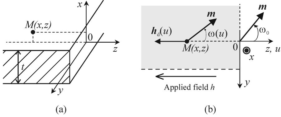
Fig. 1. (a) Geometry of the model. The semi-infinite slab corresponds to  $z < 0$ , (b) Top view of the dot.  $u$  is the dimensionless variable for  $z$
