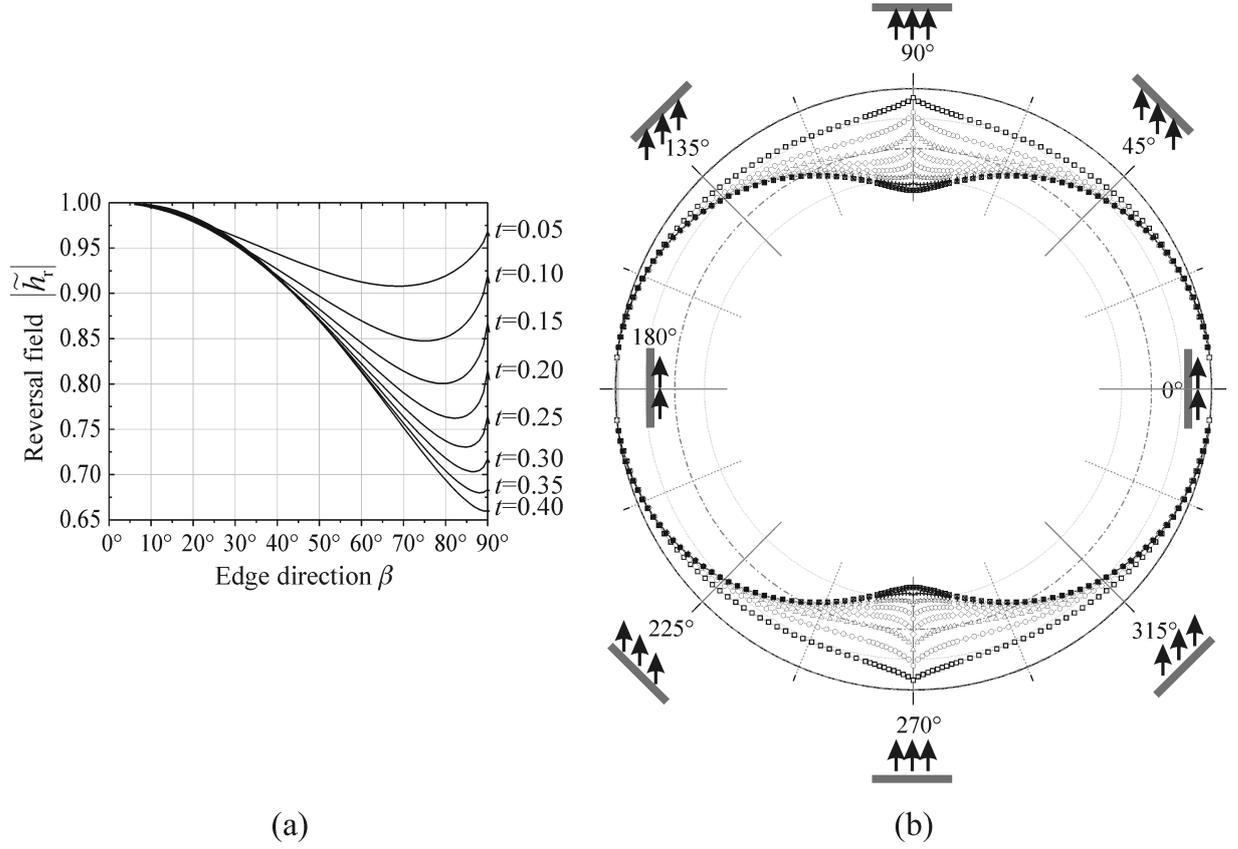
Fig. 4. Reversal field  $|\tilde{h}_r|$  predicted by the analytical model as a function of edge orientation  $\beta$  for several thicknesses  $t$ . (a) Cartesian plot, (b) Polar plot: the angle is the edge orientation  $\beta$  while the radius stands for  $|\tilde{h}_r|$ . The outer diameter stands for  $|\tilde{h}_r| = 1$ . The orientation of the easy axis with respect to the edge is sketched around the plot.
