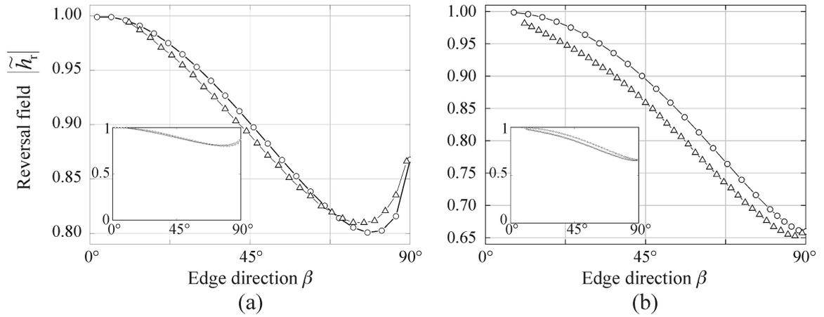
Fig. 7. Reversal field  $|\tilde{h}_r|$  predicted by the model ( $\circ$ ) and numerical simulations ( $\triangle$ ) for two thicknesses  $t = 10 \text{ \AA}$  (a) and  $t = 27 \text{ \AA}$  (b). Insets: Same curves but with full scale. Physical parameters are:  $A = 2 \times 10^{-11} \text{ J.m}^{-1}$ ,  $M_s = 1.73 \times 10^6 \text{ A.m}^{-1}$ ,  $K = 4.76 \times 10^5 \text{ J.m}^{-3}$ .
