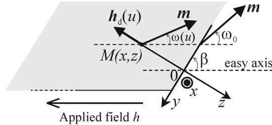
Fig. 3. Top view of the extended geometry of the new model: the edge is tilted by an arbitrary angle  $\beta \neq 90^\circ$  with respect to the easy axis.
