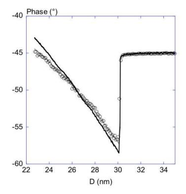
FIG. 5: Experimental phase variation (open black circles) versus tip-surface distance and its comparison with theoretical curves deduced from the long relaxation times model,  $A^{-5/2}$  equ.5 (continous grey line) and the short relaxation times model,  $A^{-3/2}$  equ.4 (continuous black line). The experimental parameters are  $A_{free} = 36$  nm ( $A_0 = 51$  nm) and time = 7 hours.
