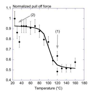
FIG. 7: Evolution of the normalized pull off force as a function of the silica sample temperature deduced from Contact mode experiments<sup>36</sup>. The normalization pull off force is 82 nN. The black line is a guide line for eyes. The arrows 1 and 2 indicate the time-temperature equivalence that can be extracted by comparing the Tapping mode and Contact mode experiments (see text and fig.6).
