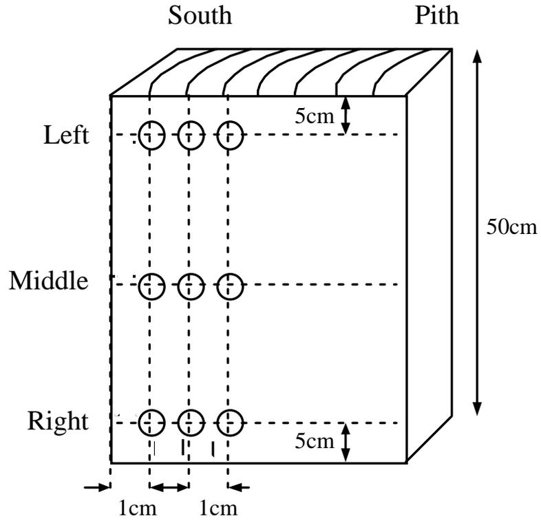
Figure 1: Schematic localisation of measurement points for boards
