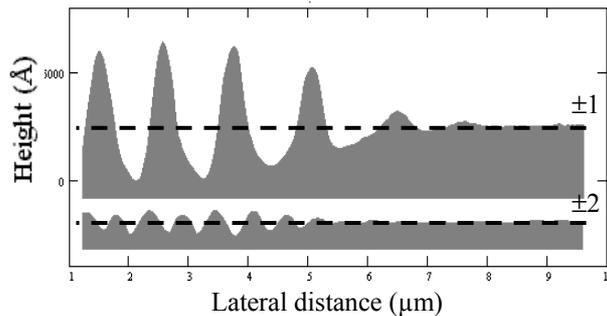
**Fig.3** AFM profile of the edge of the KrF ablated patterns  $p=2.1 \mu\text{m}$  on PEN showing the rise of transient liquid above the original surface level (horizontal dotted line). Upper profile is for the experiments with  $\pm 1$  order beams and lower one for  $\pm 2$  beams.
