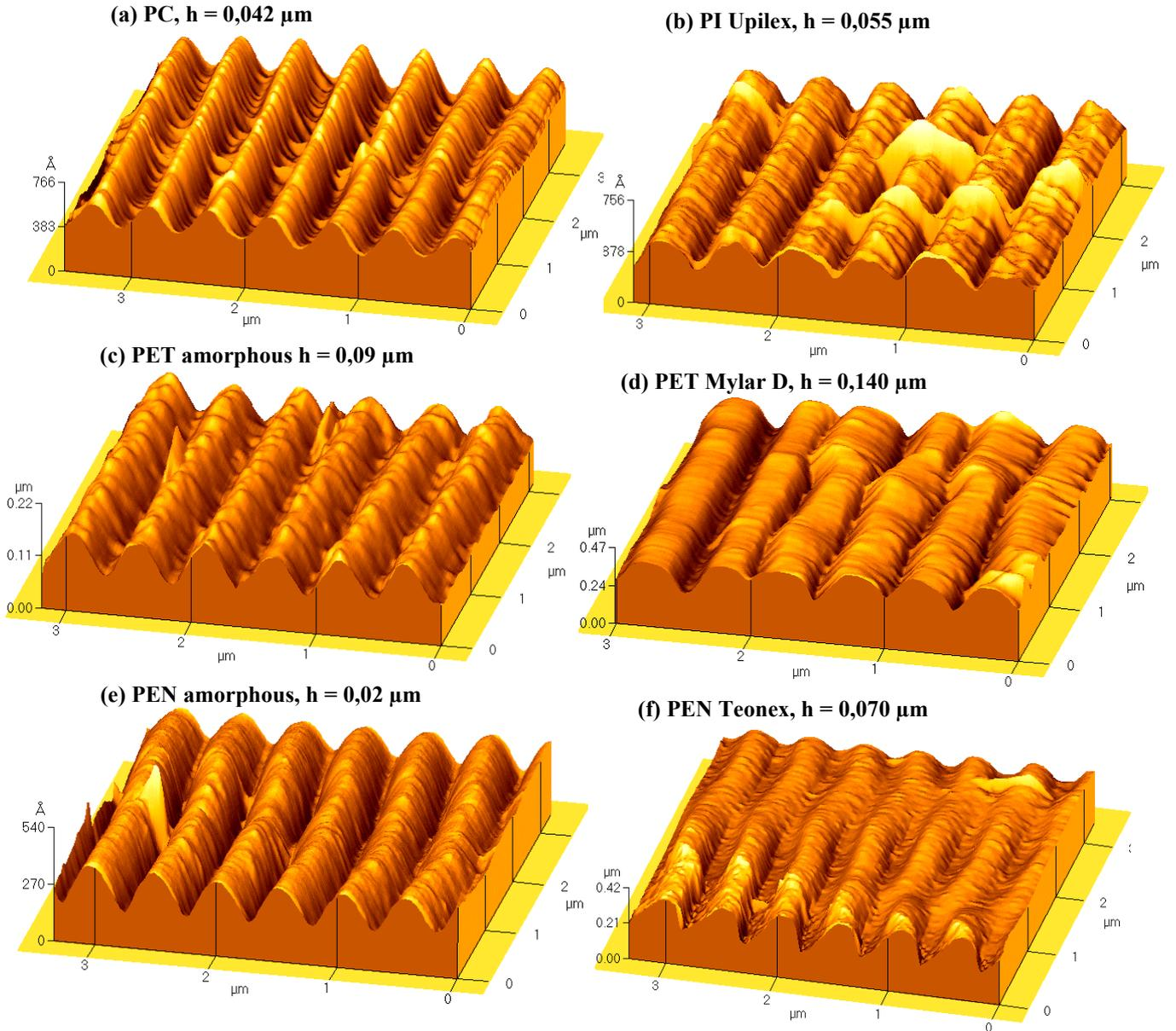
**Fig.2** KrF laser ablation patterns obtained with the 2 beams filtering experiments described in 2.1, by using diffracted beams of orders  $\pm 2$ . The obtained period is  $0.53 \mu\text{m}$  which corresponds to  $p/4$  where  $p=2.1 \mu\text{m}$  is the period of the normal grating image (the spatial period is quadrupled).
