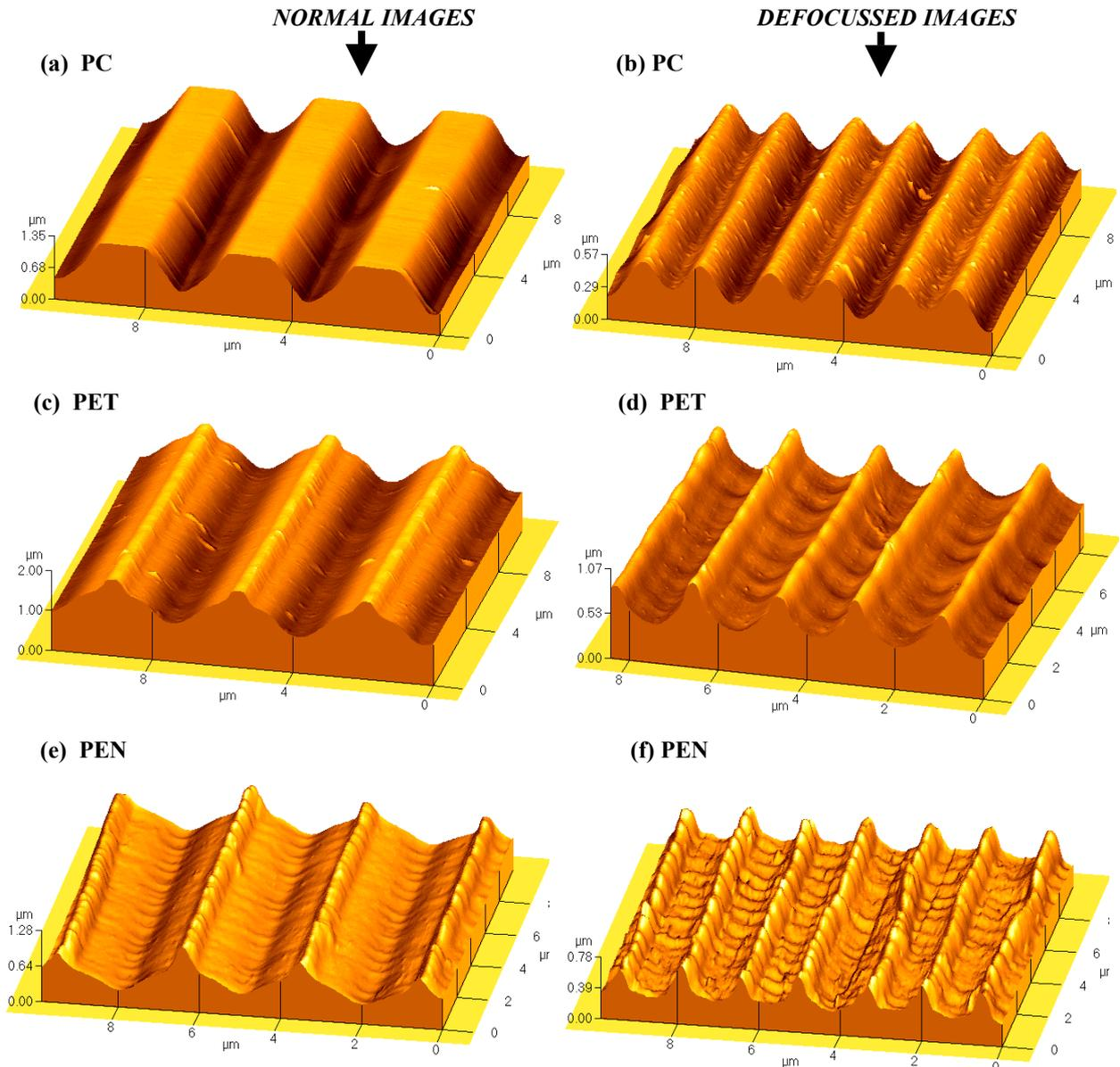
**Fig.1** KrF laser ablated patterns by projection with a precision lens and measured by AFM. Defocussing experiments ( $z_{1/2}$ ) images displaying a double spatial frequency for PC, PET and PEN (b,d,f) are displayed in the right-hand column. In the left-hand column (a,c,e) normal grating images for comparison. Normal periods are  $3.7 \mu\text{m}$  for PC, PET and  $3.0 \mu\text{m}$  for PEN. Irradiations were done with a single pulse of fluence  $F=1 \text{ J/cm}^2$  in air.
