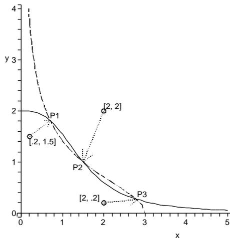
Figure 1: nullclines of system (9). (The dash line represents  $f_1(x, y) = 0$  and the solid one represents  $f_2(x, y) = 0$ ). The central equilibrium  $P2$  can be shown to be unstable while the two others,  $P1$  and  $P3$  are stable. The arrows represent the three experimentations described in the text.
