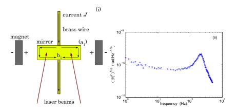
Figure 1: (i) Schematic drawing of the oscillator; (ii) FDT check in oil: the circles (o) correspond to the direct measurement of the noise and the dashed curve is  $\sqrt{\langle |\hat{\theta}|^2 \rangle}$  computed by inserting the measured response function in the FDT, Eq. (12)
