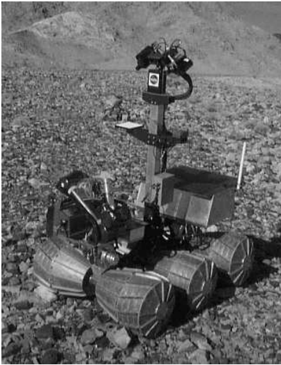
Figure 9: The Marsokhod rover
