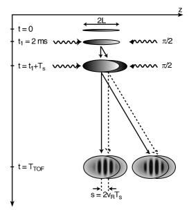
**Fig. 1.** The condensate is released from the trap at t=0 and has a half-length of L. A sequence of two Bragg pulses is applied to generate the interferometer. Two output ports are created  $(p=0,\,p=2\hbar k_{\rm L})$  with complementary fringe patterns.
