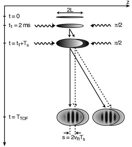
**Fig. 1.** The condensate is released from the trap at  $t = 0$  and has a half-length of  $L$ . A sequence of two Bragg pulses is applied to generate the interferometer. Two output ports are created ( $p = 0, p = 2\hbar k_L$ ) with complementary fringe patterns.
