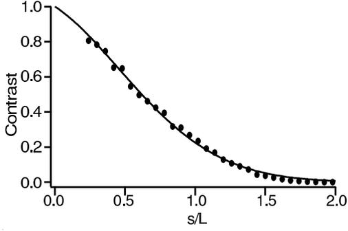
**Fig. 3.** Points represent the contrast extracted from our simulated absorption images (see text) as a function of  $s/L$ ,  $L$  being the condensate half-length, for  $T/T_\phi = 1$ . These points are fitted by the product of a gaussian and an exponential (solid line) which we take to be our theoretical effective correlation function  $C^{\text{eff}}(s)$ .
