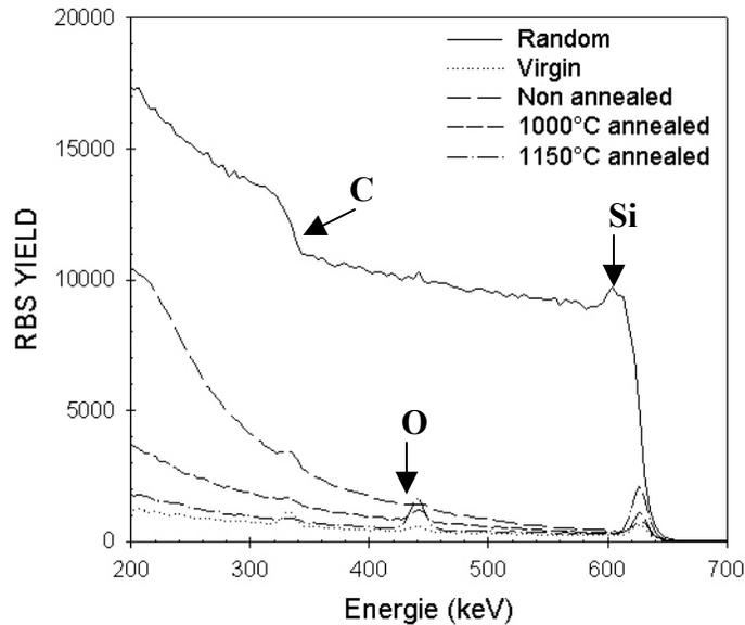
**Figure 5** : Evolution of RBS/C spectra in the thermal annealing processes implanted at RT and subsequently annealed at several temperatures.
