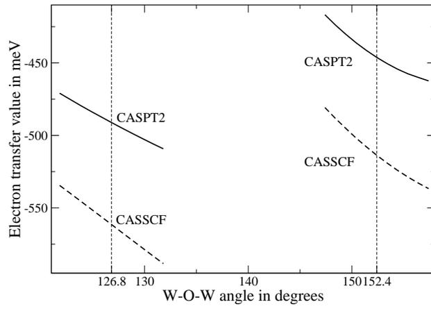
Figure 3: Variations of the value of the electron transfer parameter with the  $W - O - W$  angle around the real structure. The curves on the left represent the variation obtained from edge-sharing fragments, the curves on the right represent the variation obtained from corner-sharing fragments.
