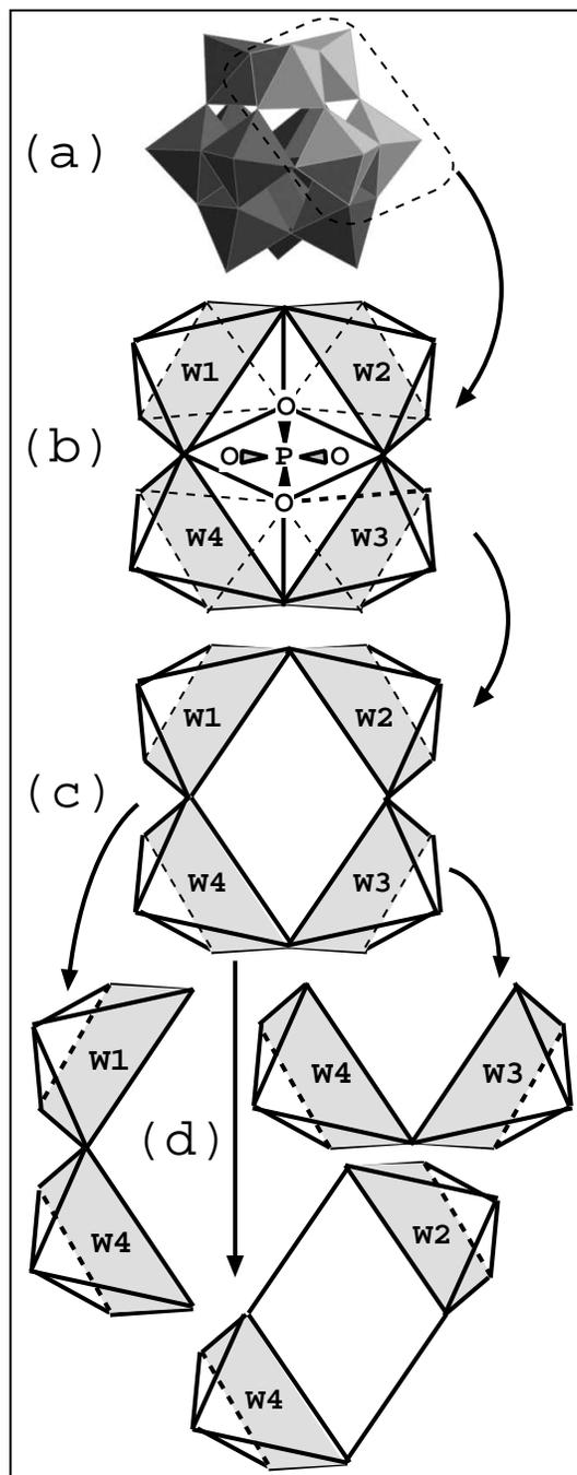
Figure 1: (a) Schematic structure of a Keggin anion. (b) The  $PW_4O_{20}$  fragment. (c) The  $W_4O_{16}$  fragment. (d) The three 2W-based fragments. The oxygen atoms occupy the corners of the octahedra or pyramids. The atoms modelled by punctual charges and TIP's are not represented.
