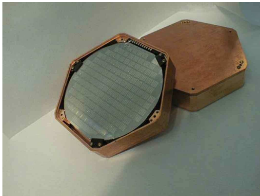
Fig. 9. Photograph of a Z-sensitive ionisation-phonon (ZIP) detector of the CDMS experiment in its mount. The photolithographically-fabricated thin film on the surface is the phonon sensor, trapping non-equilibrium phonons in Al fins. The aluminum film is coupled to tungsten sensors in the superconductor-normal transition. Silicon and germanium ZIPs, weighing 100 g and 250 g respectively, have been operated in the Stanford shallow underground laboratory and are presently operated in the Soudan (Minnesota) underground laboratory
