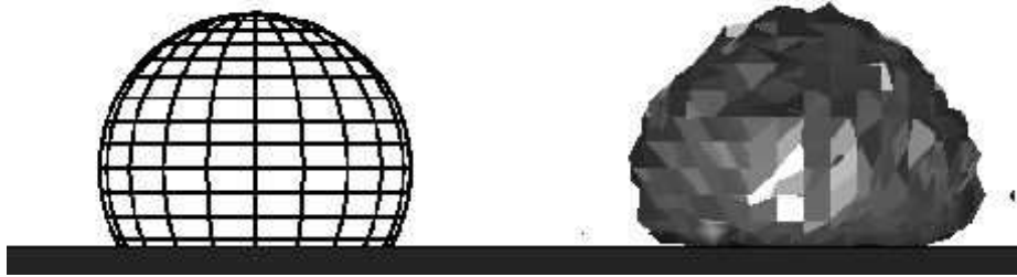
FIG. 7 – Snapshot of a liquid drop growing on a planar surface in direction [100] ( w_{mf}/w_{ff} = 0.3 , T/T_c = 0.4 , 1500 liquid sites) compared with a macroscopic drop with a 120^\circ contact angle. \kappa = 0.02 . One can check that the underlying BCC lattice does not affect the spherical shape of the bubble.
