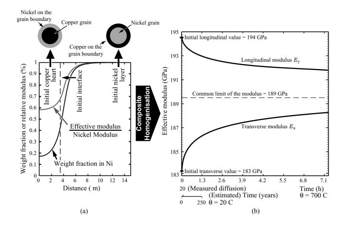
**Fig. 8.** First homogenisation step (Self-consistent scheme of a piecewise constant chemical concentration) for one half of the bilayered material, with a thicker copper layer than in Fig. 1b, for 37min of diffusion at 700°C. Effective elastic modulus vs. time for diffusion at 700°C and an estimate of the equivalent time for 20°C.
