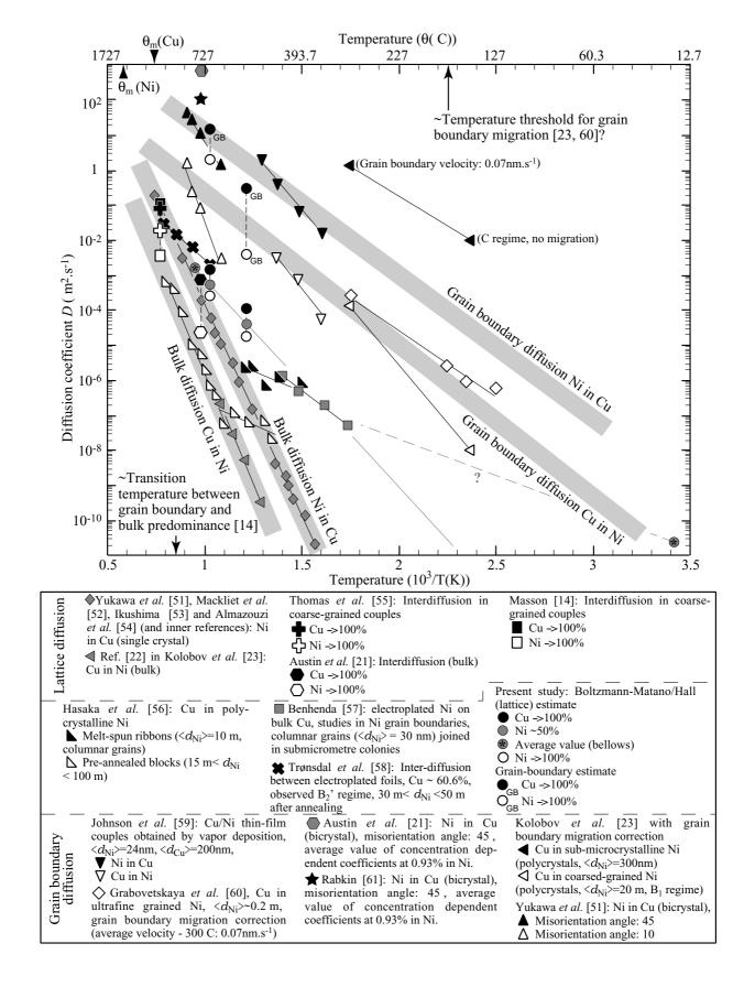
Fig. 5. Arrhenius plot for the change of global diffusion coefficients with temperature for Ni/Cu couples. All compositions are given in weight fraction,  $\theta_{\rm m}$  stands for the melting temperature. Grain boundary diffusion coefficients are plotted by assuming that the grain boundary width,  $\delta$ , is independent on the temperature and is equal to 0.5nm [42] and that the segregation factor is close to one at every temperature [27].
