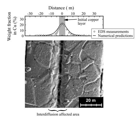
**Fig. 4.** Measured and predicted weight fraction in copper of a bellows after heat treatment at 780°C for 15min. Note the (strong) grain growth and its interaction with diffusion revealed by chemical etching [2] (SEM micrograph).
