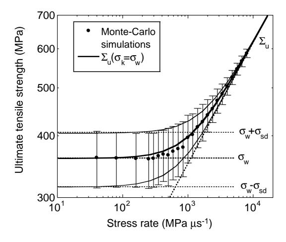
Fig. 3. Ultimate strength vs. stress rate. The dots and error bars represent results obtained by Monte-Carlo simulations (500 realizations/point) and their standard deviation for an SiC-100 ceramic. The curves are obtained by using Eqn. (25)
