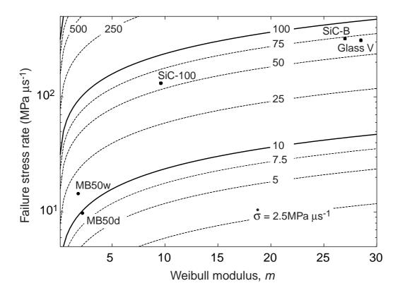
Fig. 9. Transition map [see criterion (36)] where the failure stress rate  $\sigma_{\rm w} \left(\frac{Z_{\rm eff}}{Z}\right)^{1/m} k C_0 \left(\frac{S}{Z}\right)^{1/n}$  is plotted as a function of the Weibull modulus m for different applied stress rates  $\overset{\bullet}{\sigma}$  for five brittle materials  $(n=3,\ Z=1{\rm cm}^3)$ . Above a given curve, a dynamic and deterministic solution applies. Below a given curve, a quasi-static and probabilistic solution applies.
