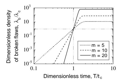
Fig. 2. Dimensionless density of broken flaws vs. dimensionless time for three different Weibull moduli m.
