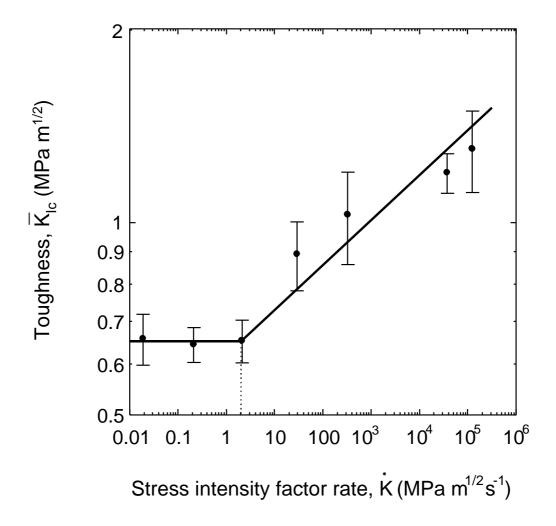
Fig. 7. Toughness vs. stress intensity factor rate for soda lime silica glass. The solid symbols are experimental data [43] and the solid lines corresponds to the prediction of the 'quasi-static' and 'dynamic' regimes [see Eqns. (30) and (34)].
