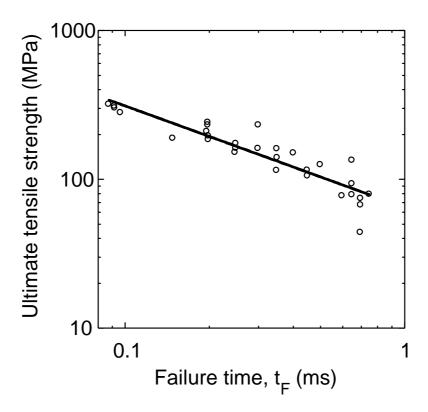
Fig. 5. Ultimate strength vs. stress rate for soda lime silica glass. The open symbols are experimental data [42] and the solid line corresponds to the prediction of the 'dynamic' regime [see Eqn. (15)].
