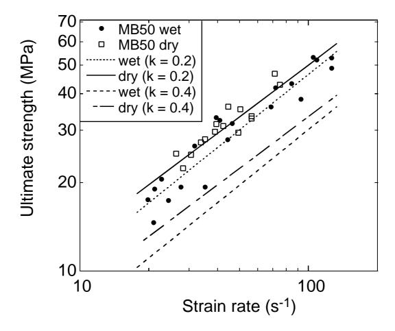
Fig. 4. Ultimate strength vs. stress rate for dry and wet MB50 concrete measured by Klepaczko and Brara [40] and predicted by using two different values of the cracking velocity factor k.
