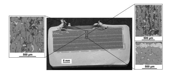
Fig. 3. View of a multilayered armor made of R-SiC-Al ceramics impacted by an AP 7.62 mm bullet. No perforation can be observed and the fragmentation process is confined around the impact zone (see zooms of three different zones).
