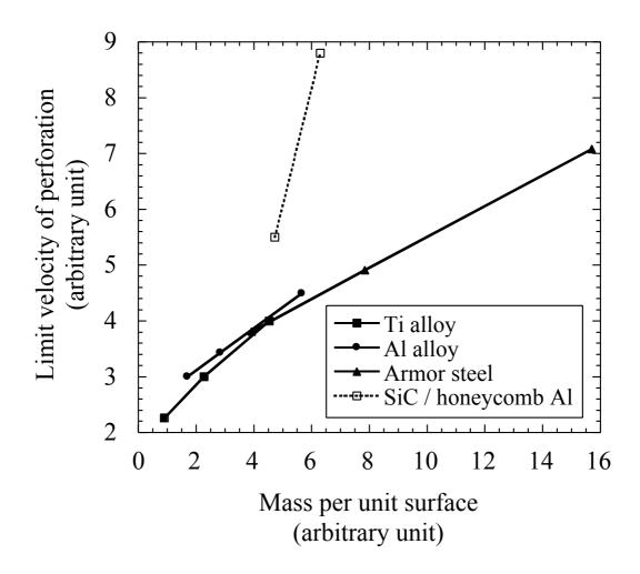
Fig. 1. Limit velocity of penetration vs. mass per unit surface of armor for different materials (after Ref. [2]).
