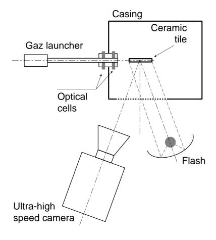
Fig. 4. Experimental configuration for EOI experiments.
