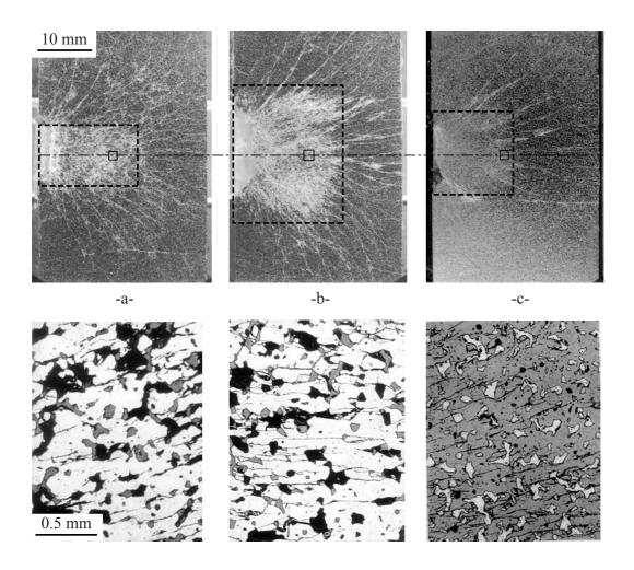
Fig. 6. Post-mortem observations and zoom around a central zone located 13 mm from the impact point:
