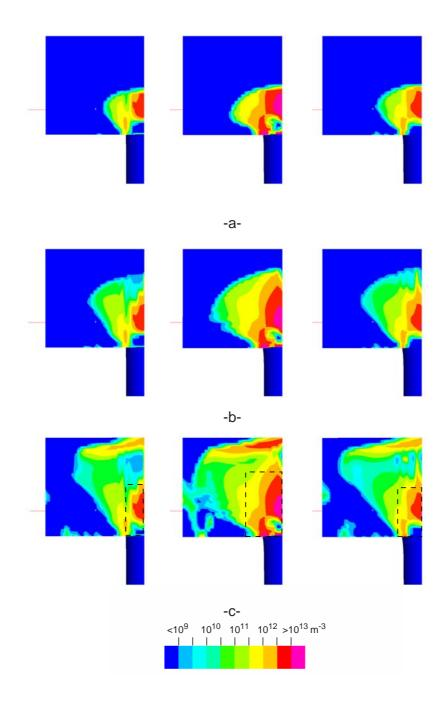
Fig. 8. Change of the cracking density with time:  $t=2~\mu s$  (a),  $t=3~\mu s$  (b),  $t=4~\mu s$  (c) after impact for R-SiC impacted at 100 m/s (left) and 200 m/s (middle), R-SiC-Al impacted at 200 m/s (right).
