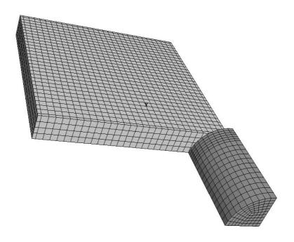
Fig. 7. Mesh of one quarter of a ceramic tile and a striker.
