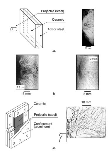
Fig. 2. a-Schematic of a normal impact on a bilayered system. Post-mortem observation of a SiC-100 ceramic / armor steel backing impacted by a steel projectile (AFNOR 100C6, AISI 52 100) at 250 m/s.
