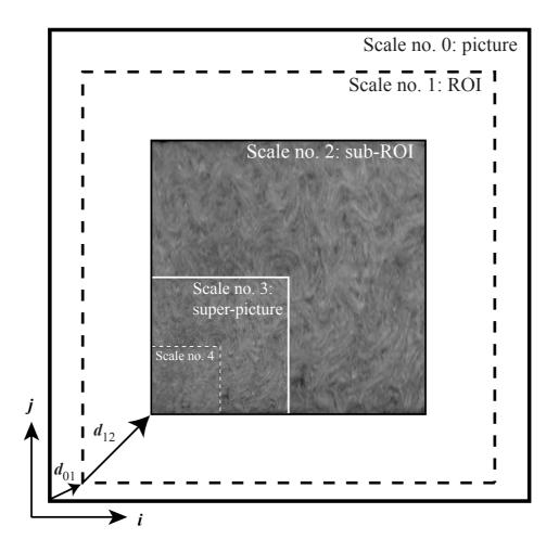
Fig. 4. Different notations used in the multi-scale approach. Sub-ROI of a reference image (scale no. 2) and corresponding super-images on scales nos. 3, 4.
