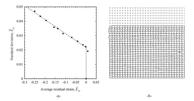
Fig. 11. (a) Average residual strain vs. standard deviation of a compressed glass wool sample. (b) Reference and deformed meshes at the end of the sequence ( $p=5, \delta=32$  pixels).
