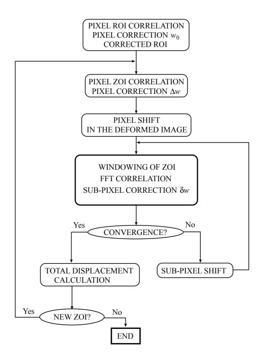
Fig. 2. Flowchart of the principal steps in a conventional correlation algorithm.
