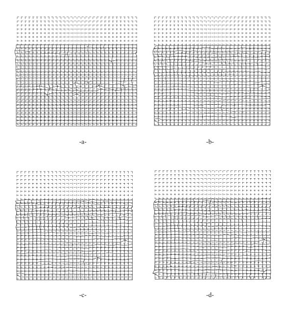
Fig. 12. Comparison of reference and deformed meshes at the end of the sequence of a compressed glass wool sample ( $p = 5, \delta = 32$  pixels). Four different options are used in the multi-scale approach: (a) no image update, (b) with image update and no iteration, (c) with image update and no limitation on  $\eta$  and (d) with image update and no test on the local texture fluctuations.
