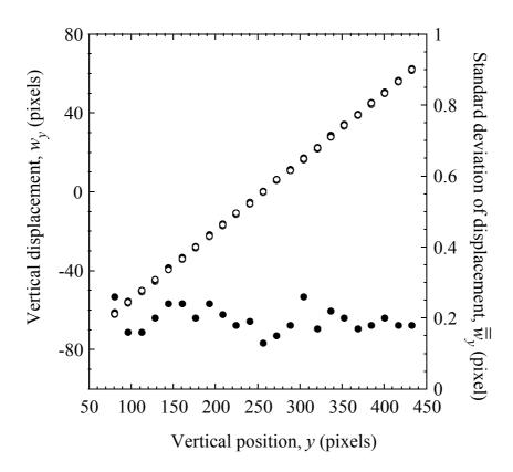
Fig. 7. Vertical displacement ( $\circ$ ) and corresponding standard deviation ( $\bullet$ ) vs. vertical position y of the ZOI when a strain  $E_{yy}=0.35$  is prescribed. The multi-scale correlation procedure is used ( $p=4, \delta=16$  pixels).
