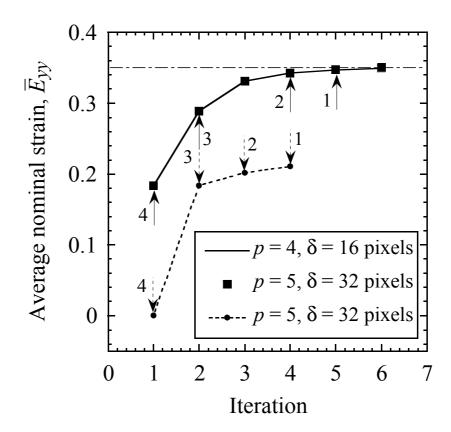
Fig. 8. Average strain vs. iteration number for different sizes  $(2^p \times 2^p)$  pixels of the zones of interest and shifts  $\delta$ . The dashed line corresponds to a simulation in which no iteration is used for a given scale. The arrows show the first time a scale, the level of which is indicated by the numbers close to the arrows, is invoked. A strain  $E_{yy} = 0.35$  is applied.
