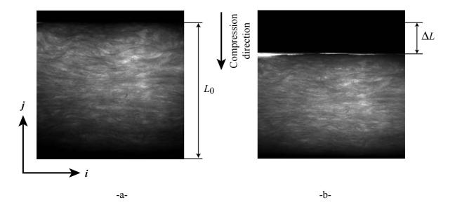
Fig. 6. Initial (a) and last 'deformed' (b) images of a glass wool sample. The reference length  $L_0$  and the length variation  $\Delta L$  are drawn.
