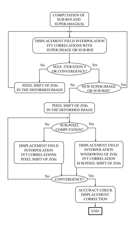
Fig. 5. Flowchart of the principal steps in the multi-scale correlation algorithm.
