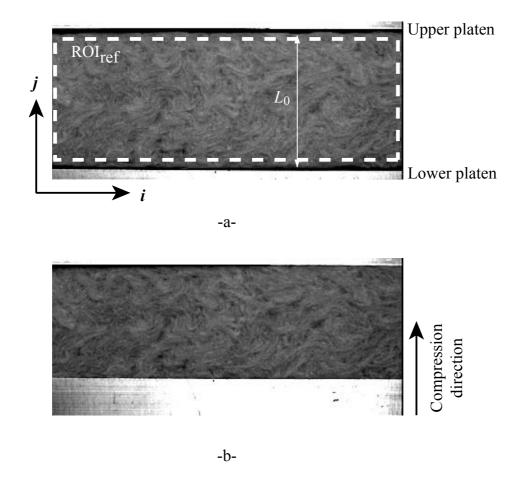
Fig. 9. Reference and deformed images of a stone wool sample. The estimated reference length  $L_0$  is drawn.
