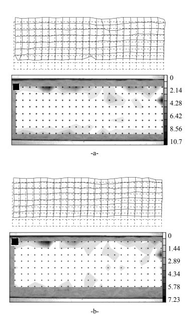
Fig. 10. Reference and deformed meshes of a stone wool sample predicted by using two strategies of the multi-scale approach and corresponding error contours: (a) no image update, (b) with two image updates. The black square depicts one ZOI  $(p=5,\delta=32~{\rm pixels})$ .
