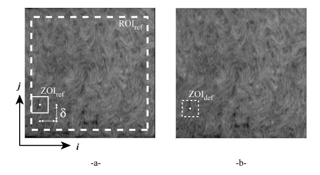
Fig. 1. (a) Initial and (b) artificially deformed ( $E_{yy} = 0.05$ ) images of a stone wool sample. The Region Of Interest ( $ROI_{ref}$ ) and two Zones Of Interest ( $ZOI_{ref}$  and  $ZOI_{def}$ ) are depicted. Four centers of ZOIs are shown on the reference picture ( $\delta$ : separation between neighboring ZOIs).
