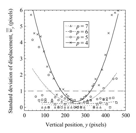
Fig. 3. Standard deviation of the vertical displacement vs. vertical position y of the ZOI when a strain  $E_{yy}=0.05$  is prescribed (Fig. 1). A classical digital image correlation procedure is used for different sizes  $(2^p \times 2^p \text{ pixels})$  of the zones of interest  $(\delta = 16 \text{ pixels})$ .
