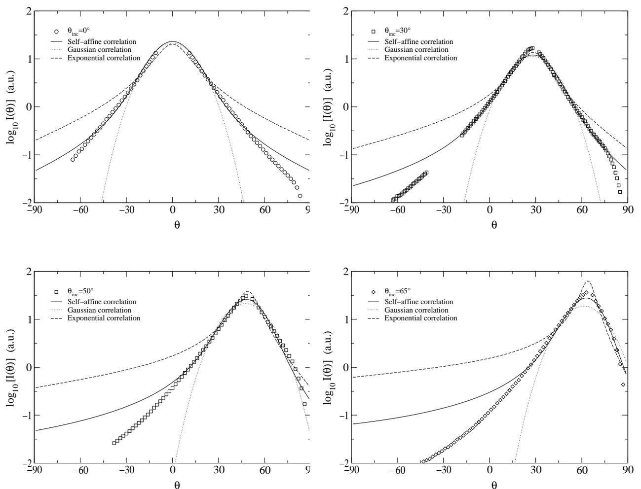
FIG. 2: Scattered intensity measurements obtained at incidence angles  $\theta_0 = 0, 30, 50$  and  $65$  degrees respectively. The experimental results are shown in symbols. The solid/dotted/dashed lines correspond to the expressions obtained for a Kirchhoff approximation in case of self-affine/Gaussian/exponential correlations respectively.
