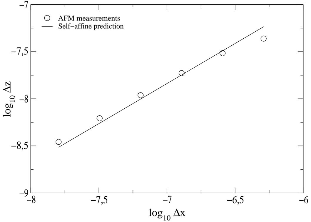
FIG. 3: Roughness analysis computed from AFM measurements (circles) compared with predictions obtained *via* a fit of the angular scattered intensity distribution assuming self-affine correlations. The slope of the line is  $\zeta = 0.78$
