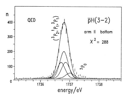
Figure 7: High-resolution spectrum of antiprotonic hydrogen [56]. The difference between the measured line shape and the solid line is due to the fact that the solid line represents a line-shape model without strong interaction, evaluated following the method described in the text (2).
