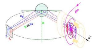
Figure 5: Principle of X-ray spectrocopy of exotic atoms with the cyclotron trap and a spherically curved crystal spectrometer. The bidimensional X-ray detector is a 6-chips cooled CCD detector and is located on the Rowland circle of radius R/2, where R is the radius of curvature of the crystal ( $\approx 3$  m)
