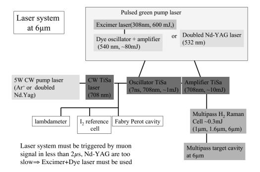
Figure 4: Principle of the  $6\mu$ m laser for the study of the muonic hydrogen  $2s\rightarrow 2p$  transition
