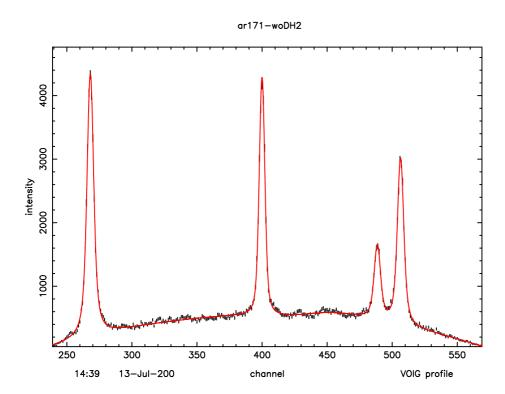
Figure 6: High-statistic X-ray spectrum from the  $1s2s^3S_1 \rightarrow 1s^2 \, ^1S_0$  transition in helium-like argon (center line) from the PSI Electron-Cyclotron Resonance Ion Trap. 37500 counts were accumulated in this line in 35 min, using the instrument in Fig. 5. The width of this 3.1 keV line is 0.4 eV. The line on the left is from  $Ar^{14+}$  and those on the right are from  $Ar^{15+}$ .
