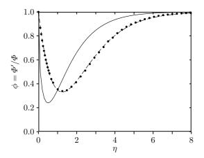
Fig. 3. Fraction  $\phi(\eta) = \Phi'/\Phi$  of remaining atoms after evaporation by one antenna, as a function of the evaporation parameter  $\eta$ . Solid line: Harmonic confinement; dashed line: Linear confinement,  $\phi$  being calculated with the approximation (11); dots: Linear confinement,  $\phi$  being calculated by a Monte-Carlo simulation.
