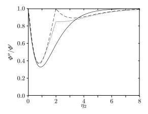
Fig. 12. Fraction  $\Phi''/\Phi'$  of the flux remaining after the second antenna as a function of its parameter  $\eta_2$ . The first antenna is driven at a frequency  $\nu_1 = \eta_1 k_B T/h$  with  $\eta_1 = 2 = 1.6\eta^*$ . The dashed line corresponds to the collisionless regime; the dotted line to a mean number of collisions between antennas  $N_c = 1.1$ ; the solid line to full rethermalization. These curves are calculated with a numerical simulation, in the case of a linear confinement.
