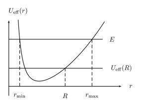
Fig. 1. Effective potential  $U_{\text{eff}}(r)$ . An atom with  $E \ge U_{\text{eff}}(R)$  is evaporated.
