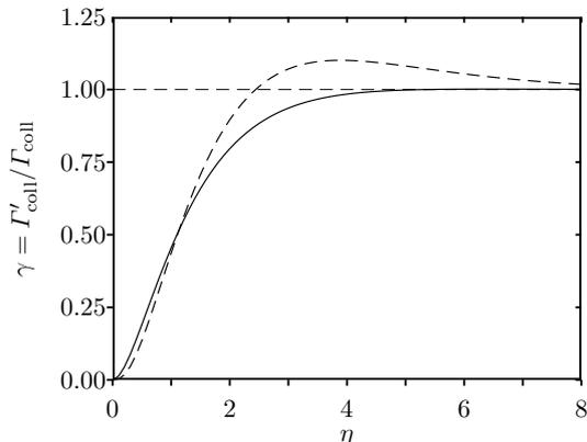
**Fig. 10.** Variation of the collision rate after evaporation by one antenna and rethermalization, as a function of  $\eta$ , for the multi-radii evaporation scheme. Solid line: harmonic confinement; dashed line: linear confinement.
